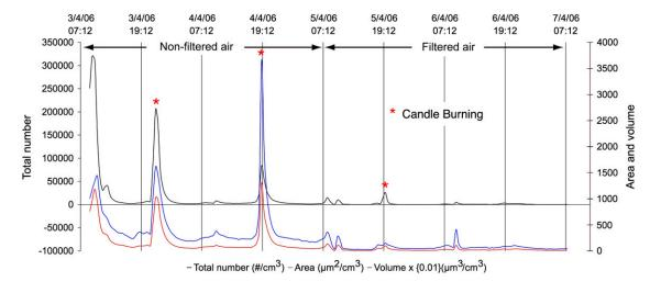
Figure 1. Number concentration (NC<sub>10-700 nm</sub>; black line), Area<sub>10-700 nm</sub>; (red line), and Volume<sub>10-700 nm</sub>; (blue line) of particles during 48 hours without and 48 hours with filtration of the indoor air in one of the included homes. Peaks in NC<sub>10-700 nm</sub> (asterisks) occurred during candle burning and cooking, as indicated.
